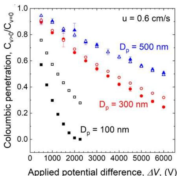
**Figure 2.** Coulombic penetration as a function of applied potential difference at a constant mean velocity  $u = 0.6$  m/s for three particle diameters:  $D_p = 100$  nm (black),  $D_p = 300$  nm (red),  $D_p = 500$  nm (blue). Filled symbols are for experiments and open symbols for simulations.
