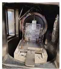
Figure 3. A contaminated PC sheet in the thermal degradation zone. On the right of the figure, we can see a protective mask which isolates the sample from the heat flow before the start of the test
