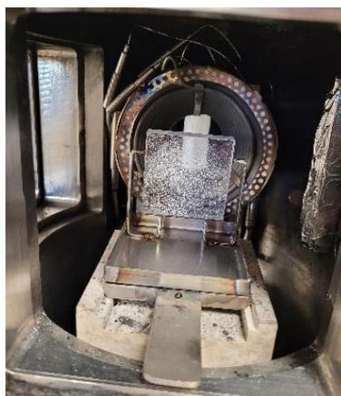
Figure 3. A contaminated PC sheet in the thermal degradation zone. On the right of the figure, we can see a protective mask which isolates the sample from the heat flow before the start of the test
