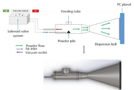
Figure 2. Schematic description of the powder dispersion apparatus
