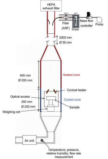
Figure 1. Schematic representation of the thermal degradation device used to assess the ARF
