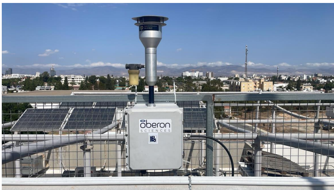
Figure 1. Aerotape instrument with a PM10 head on the roof of the Cyprus Institute in Cyprus
