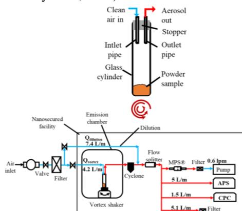
Figure 1. The vortex shaker experimental setup.
