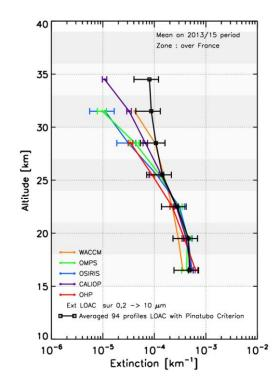
Figure 2. Comparative satellites, model, ground lidar and LOAC extinctions averaged over 3 km bands over France for the 2013-2016 period.
